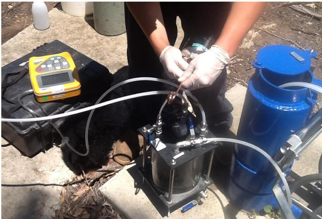
Figure 15 Example of gas collection and sampling procedure in the field
