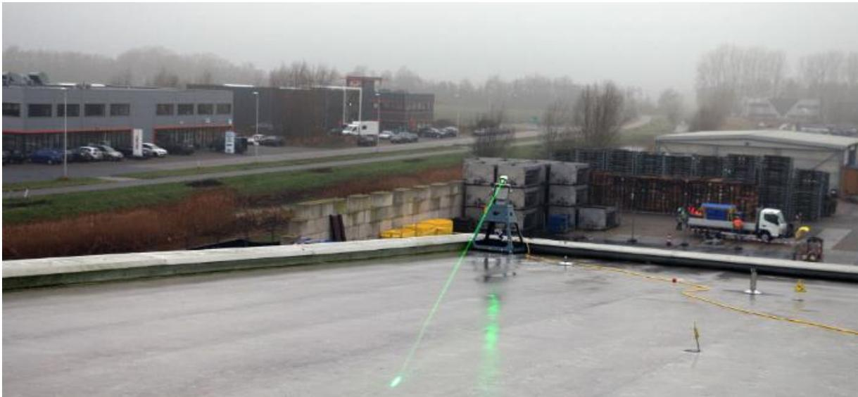
Figure 16: Bird laser deterrent in operation
