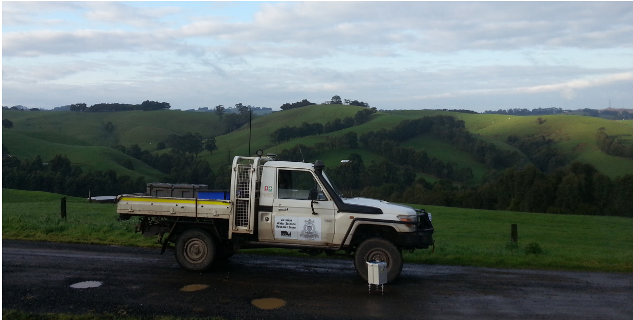
Figure 5 Gravity acquisition by vehicle
