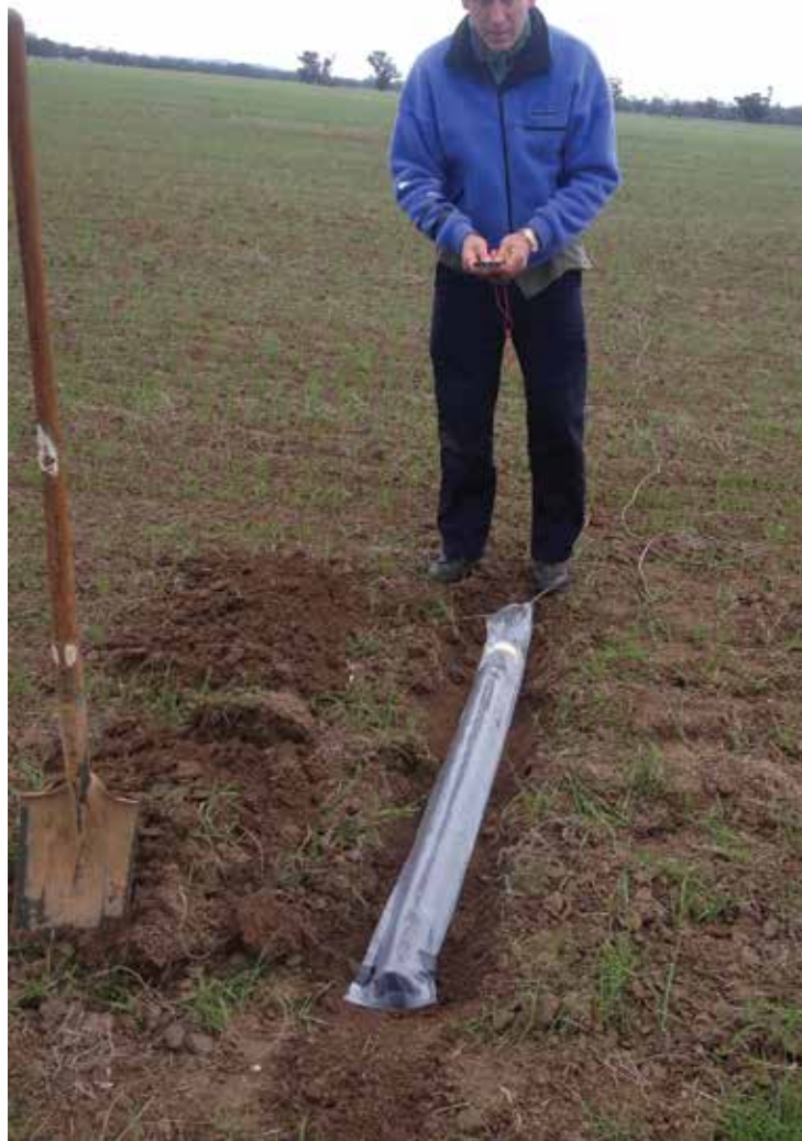
Figure 4 . Installing a horizontal magnetic sensor in western Victoria. Photo: University of Adelaide.
