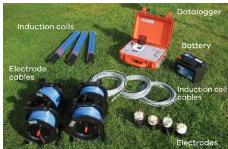
Figure 2. Magnetotelluric survey equipment. Photo: Geological Survey of Finland.
