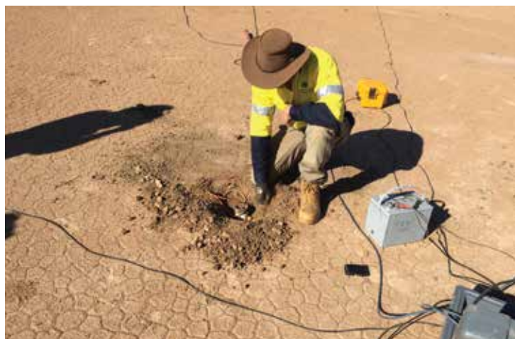
Figure 3. Installation of electrode with wires ready for connection to data logger. Photo: Geoscience Australia.
