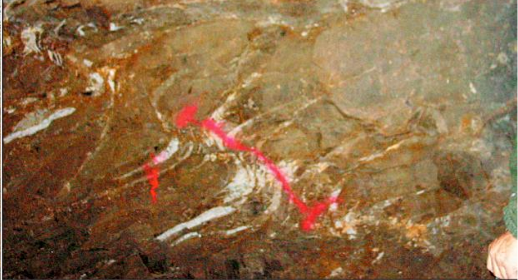
Lauraville dyke sigmoidal quartz arrays define opening under west/east reverse shear
