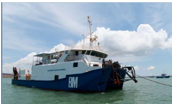
Figure 3-1: The "Bhagwan Samson Explorer" - typical vessel for pipeline surveys
