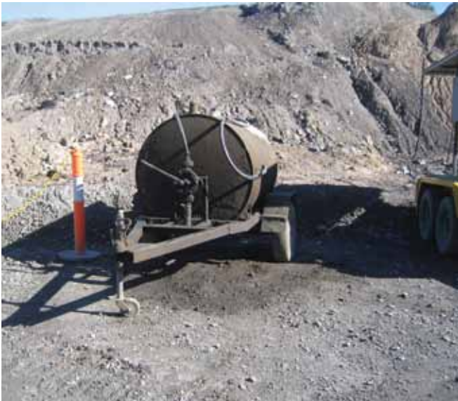
Fuel spill beneath a mobile fuel storage tank.
