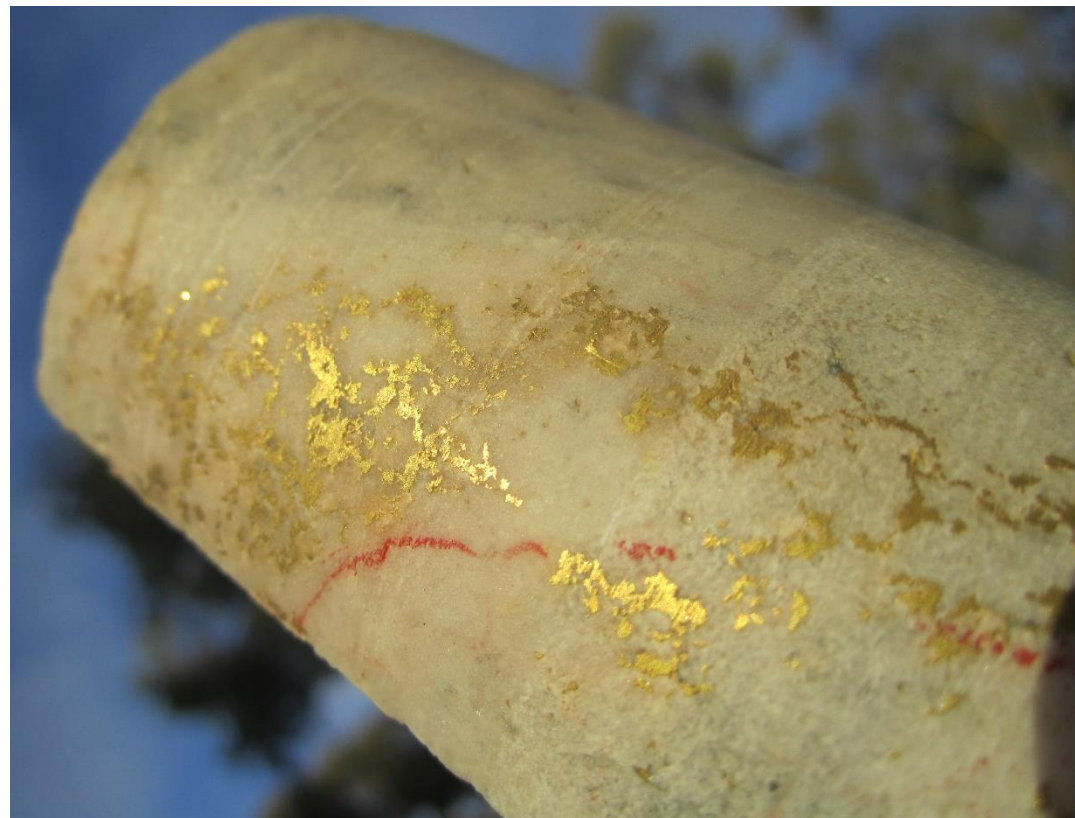
Fosterville: Lower Phoenix Fault - Eagle ore body, drill hole UDH1501: 12.5m @ 500.7 g/t Au (4.5m ETW)
