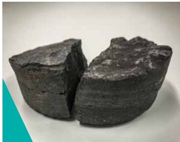
Figure 7: Seal rock – mudstone (Belfast mudstone, sample from Port Campbell-2)
