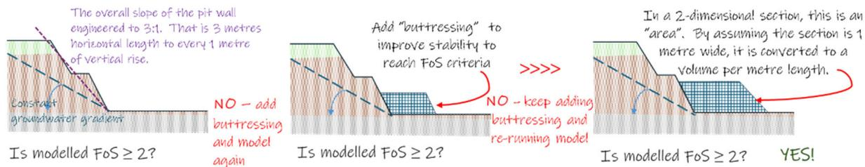
"Buttressing" – earth material placed and compacted against the pit wall to increase stability
