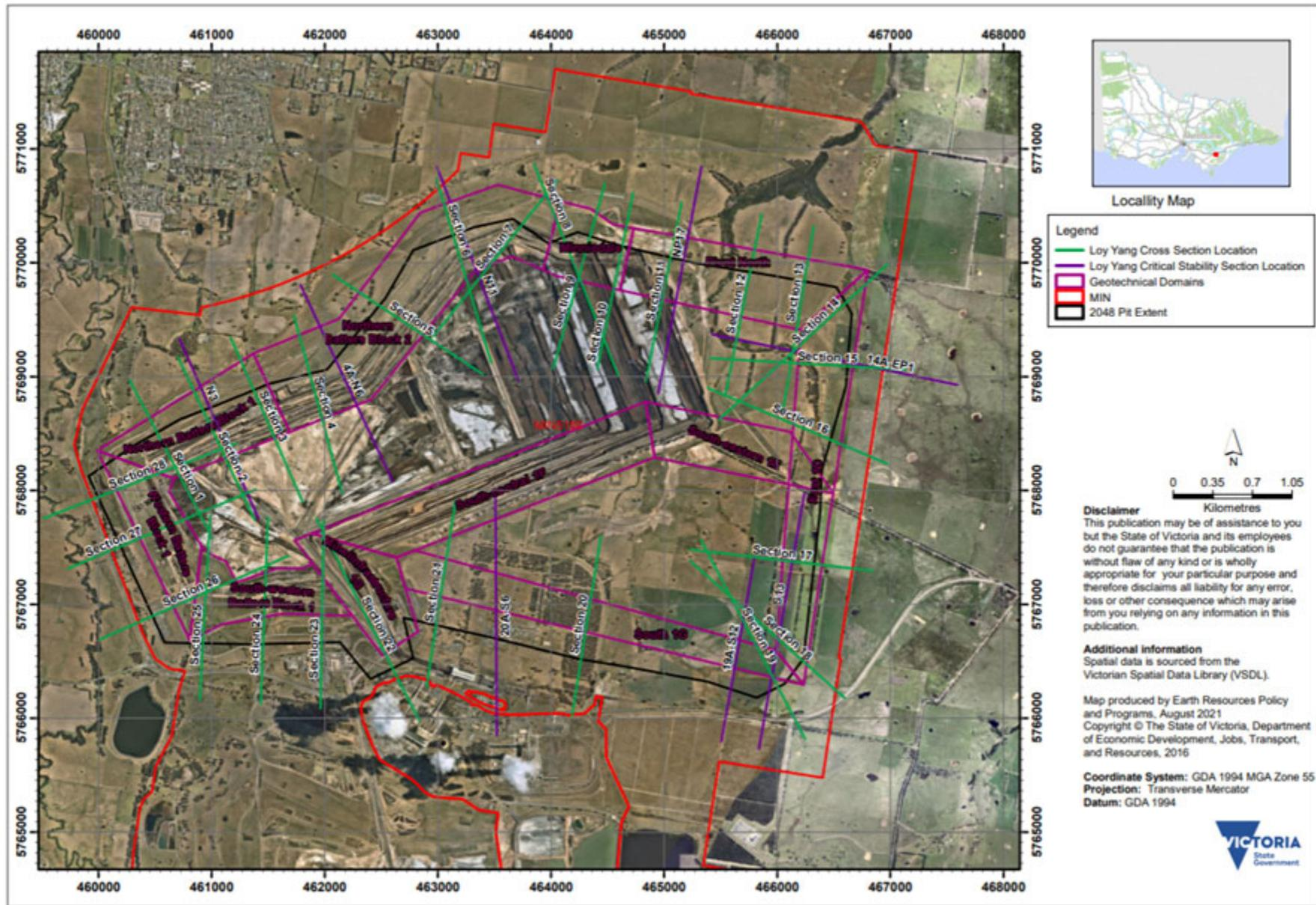
Figure 1.3 Loy Yang Mine - modelled cross section locations
