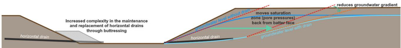
Figure 1.4 Groundwater gradients
