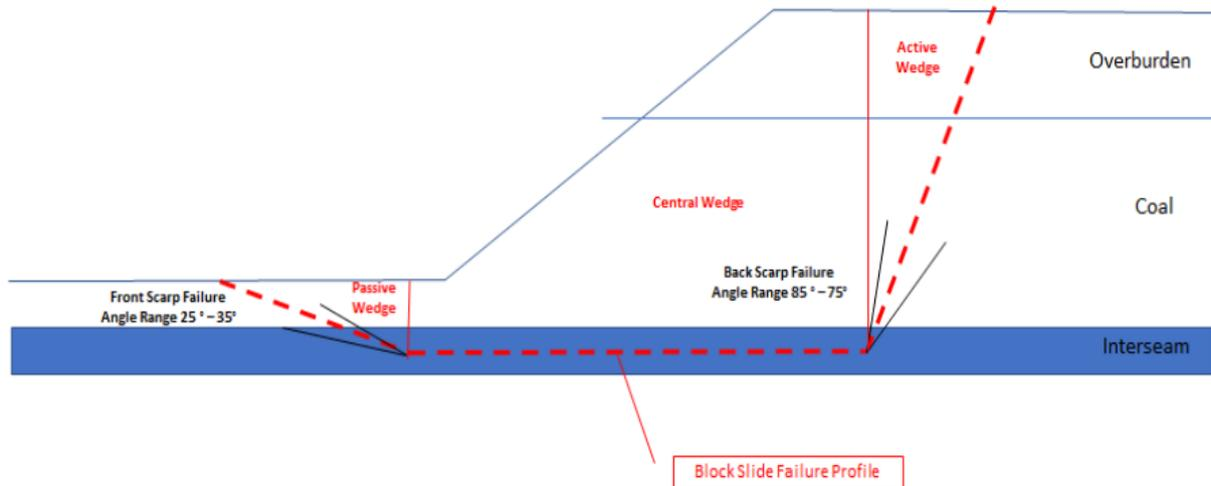
**Figure 1.7 Block slide mechanism modelled in Slide2**
