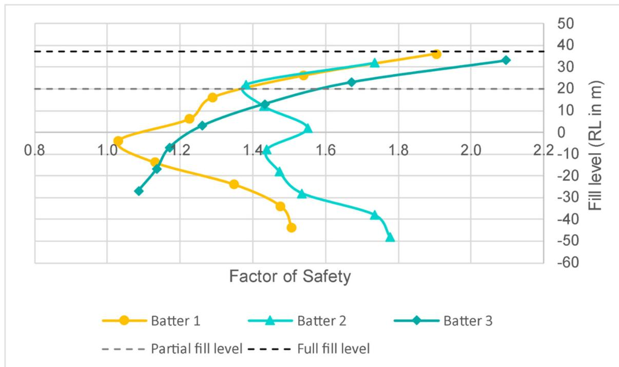
**Figure 2.2 FoS vs fill level for three different batters. NB: This graph is indicative only and does not intend to display actual values.**
