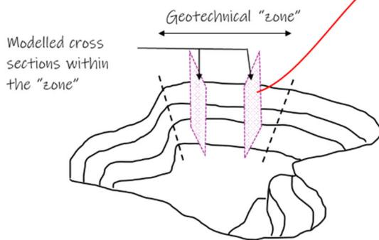
Each section used to create a mathematical "model" to test stability.
