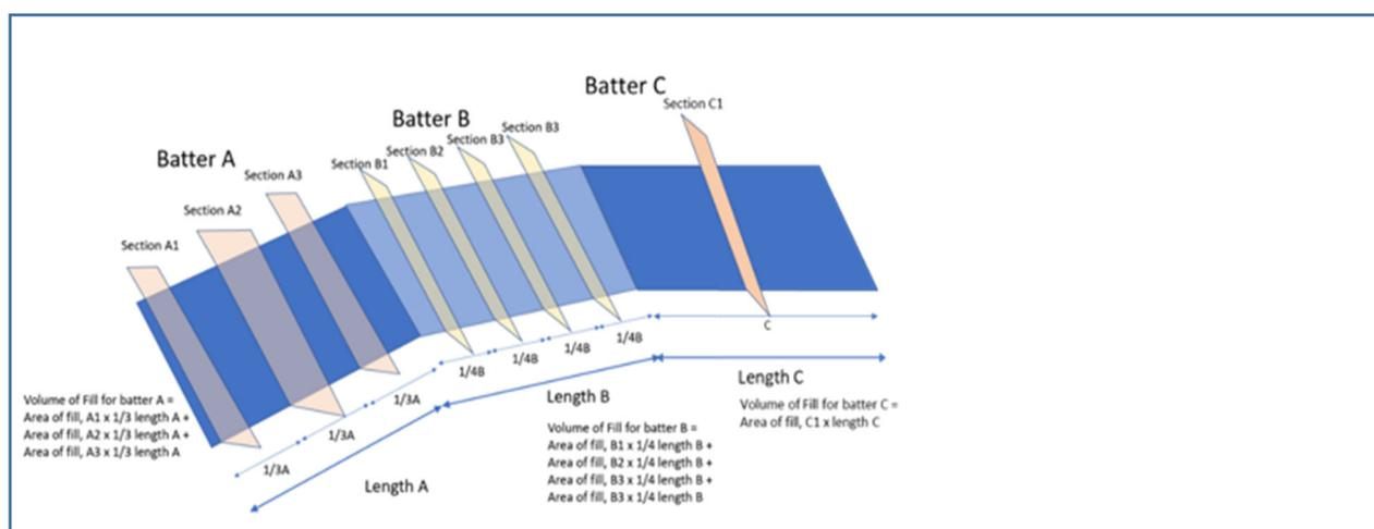
**Figure 3.2 Approach to estimating structural earthworks volumes from available geotechnical sections.**
