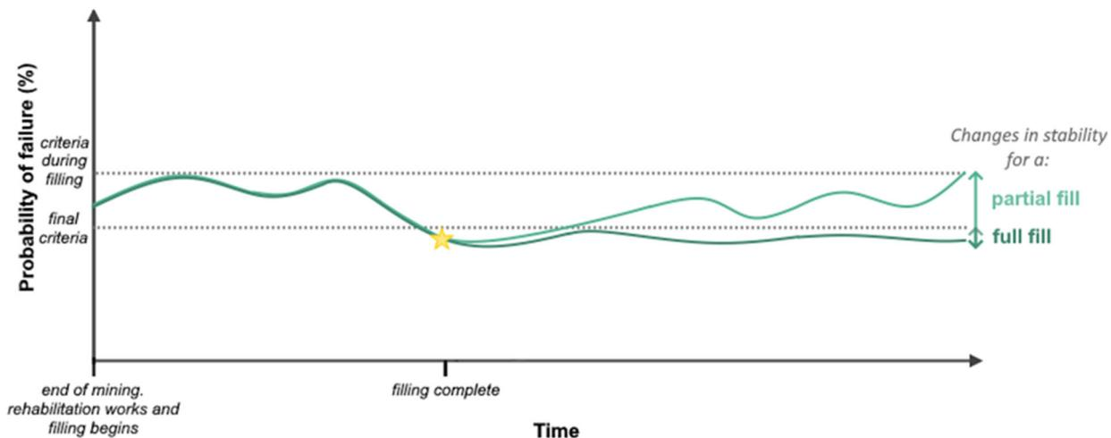
Figure 2.3 Stability changes over time for each fill option (indicative only, does not display actual values)
