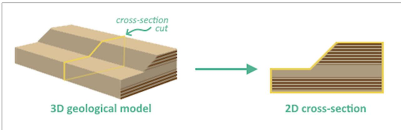
**Figure 3.1 Generation of 2D cross-sections from a 3D geological model**
