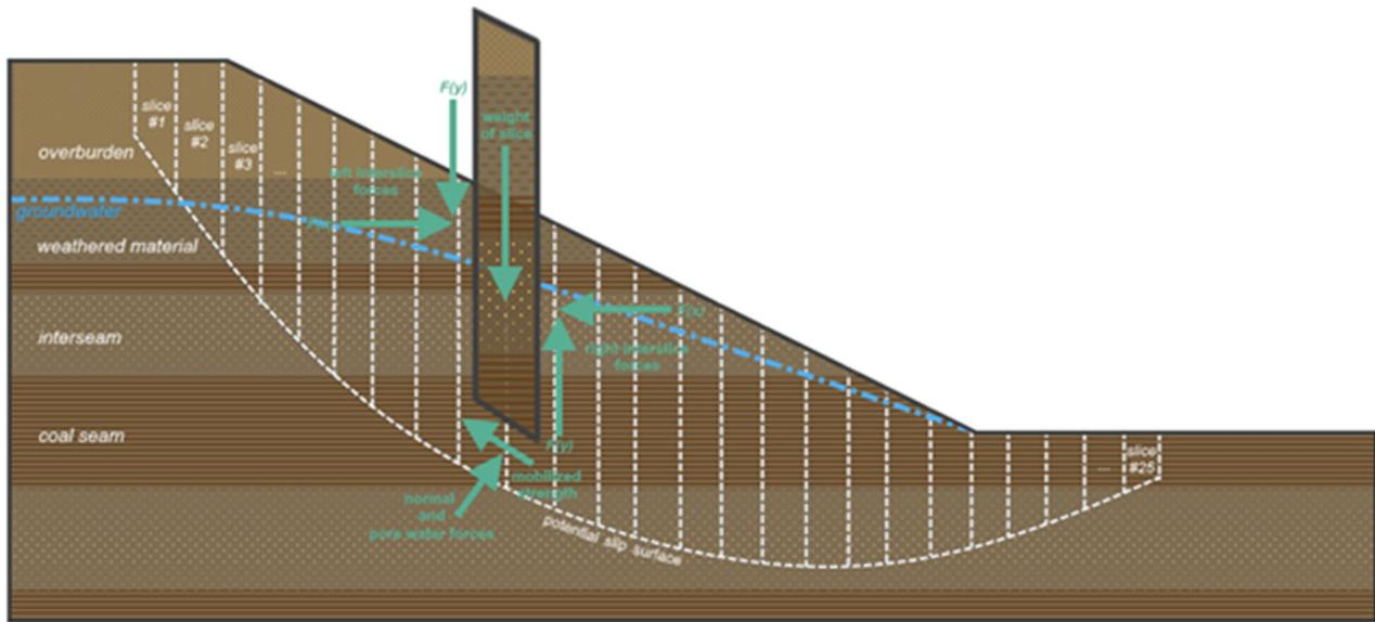
Figure 1.5 Methods of slices in limit equilibrium slope stability analyses
