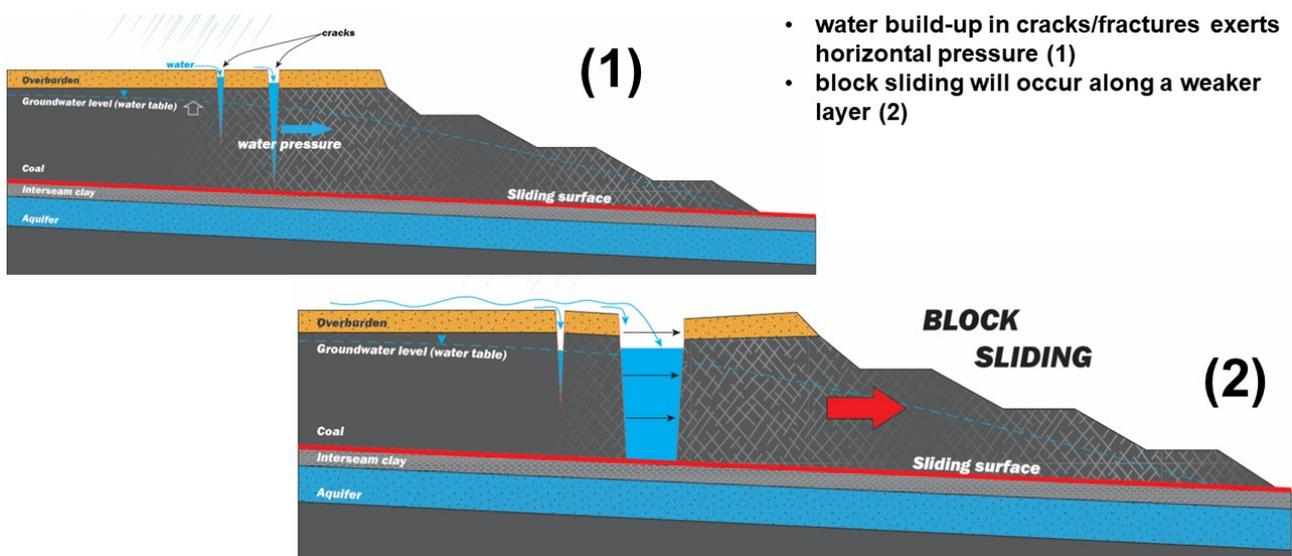
Figure 1.1 Schematic diagram of a block sliding failure mechanism in coal (courtesy MLRA)
