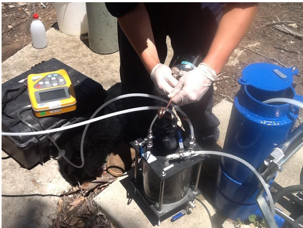
Figure 21 Example of gas collection and sampling procedure in the field
