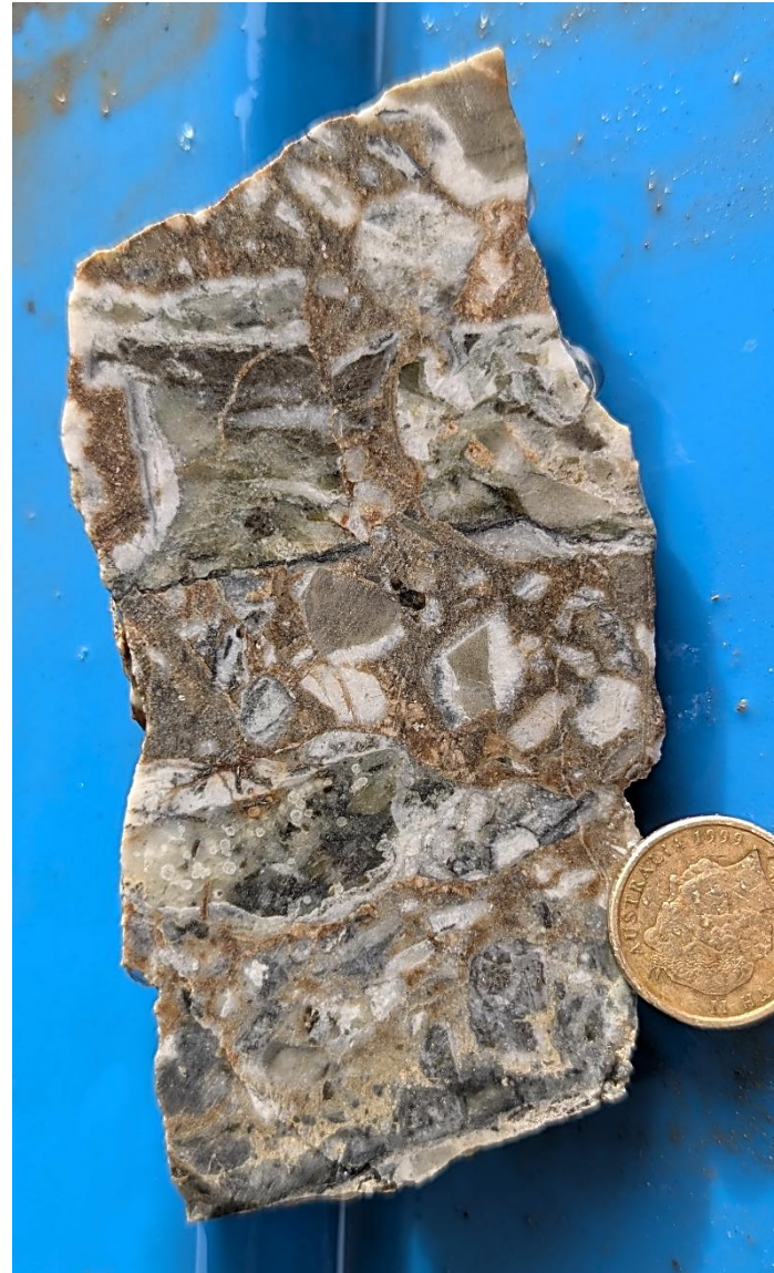
Low sulphidation breccia, moss, colloform & chaledonic quartz, ginguero banding – Nelson Creek - 2.69 g/t Au
