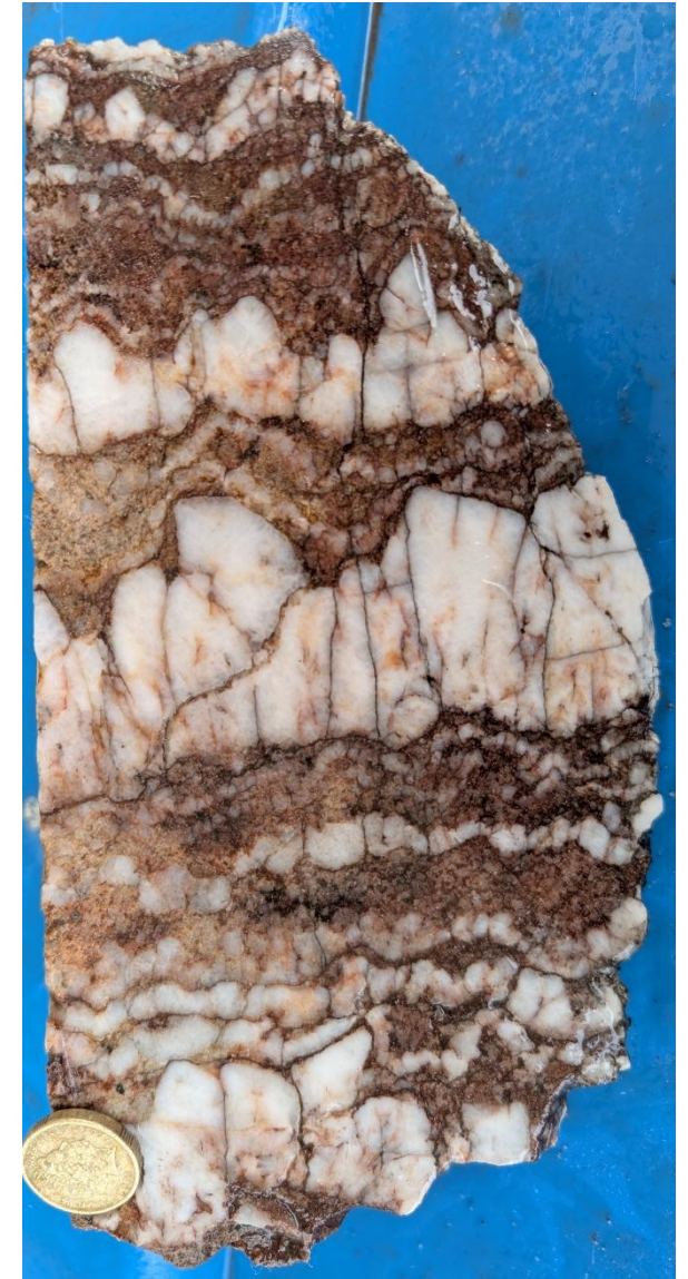
Intensely phyllic altered UST rich quartz porphyry intruding barren silicified rhyolite shoulder
