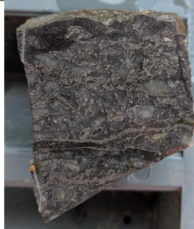
Arsenopyrite-sphalerite cemented intermediate sulphidation breccia – Gambetta – 15.4 g/t Au, 1.69 g/t Ag, 1,360 ppm Zn, 17.5 % As
