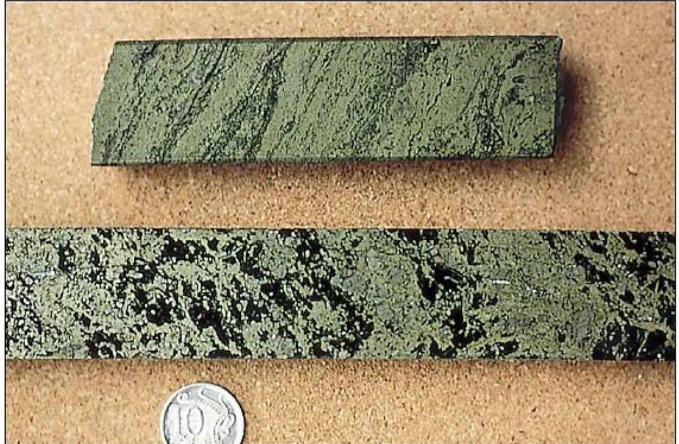
Wilga ore. Top: 20+% Cu, 1.9% Zn, 70 ppm Ag (Bend 23, 116.9 m). Bottom 13.4% Cu, 0.7% Zn, 0.2% Pb, 50 ppm Ag (Bend 19, 103 m). (VandenBerg et al., 2000. Photo by D. Barr)
