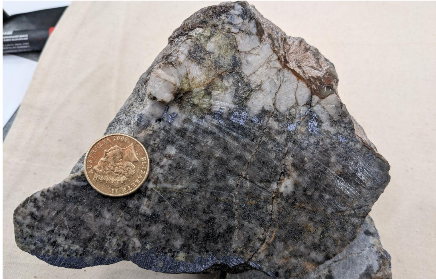
Quartz – molybdenite vein cutting intensely silicified granite with disseminated chalcopyrite – Womobi – 322316 - 1.65 % Mo, 1,265 ppm Cu, 4,520 ppm W, 4,470 ppm Sn, 3,390 ppm Bi
