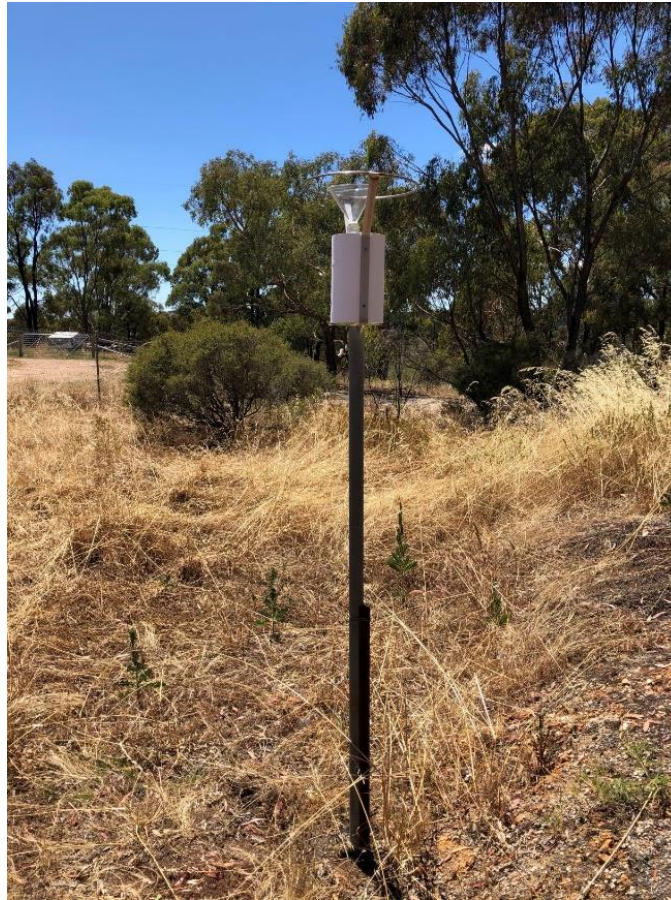
Figure 4 - Kangaroo Flat - Dust Deposition Gauge KF1 (W)
